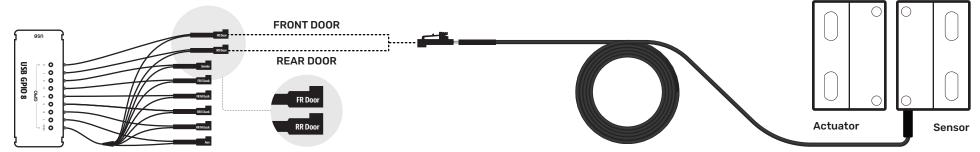
Mount sensor(s) & actuator(s) on a surface where wires can run through and won't block the door when opened. You may screw it on or use mounting tape.
